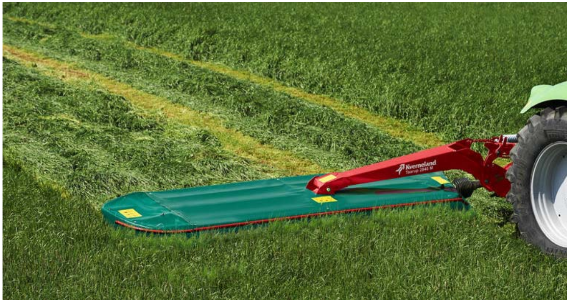
The new Kverneland Taarup 2840 M with 4.0m working width.
