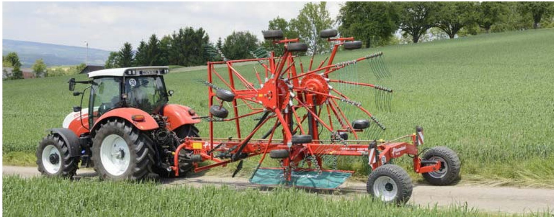
Below 4m transport height, also with tine arms mounted.
