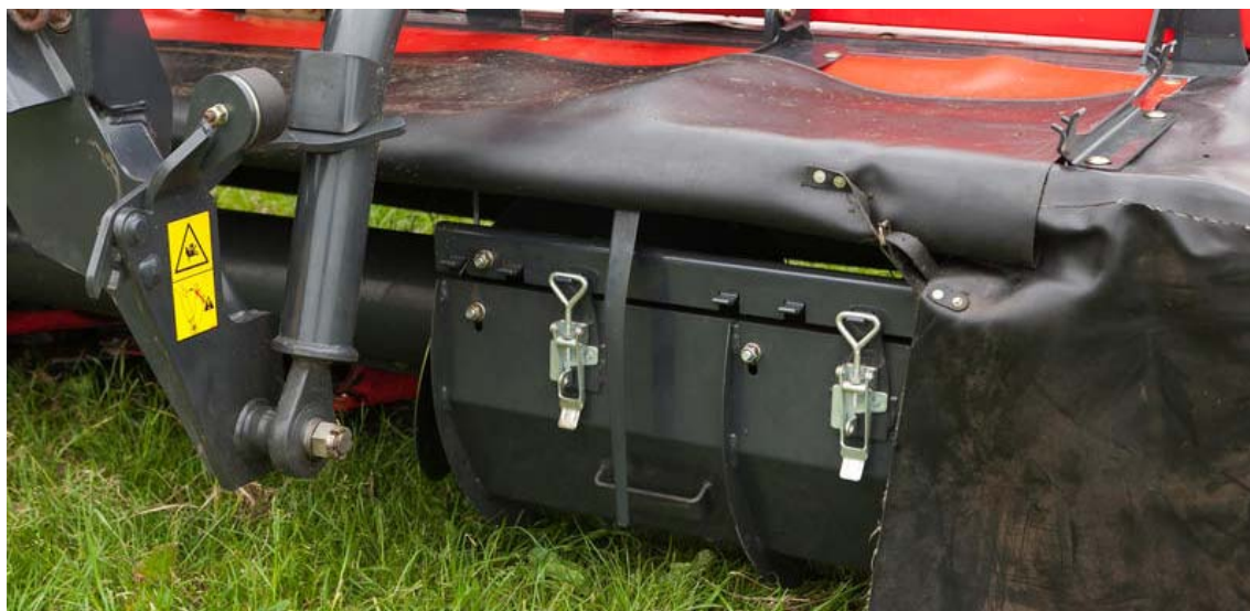
The swath is collected by the auger and guide plates.
