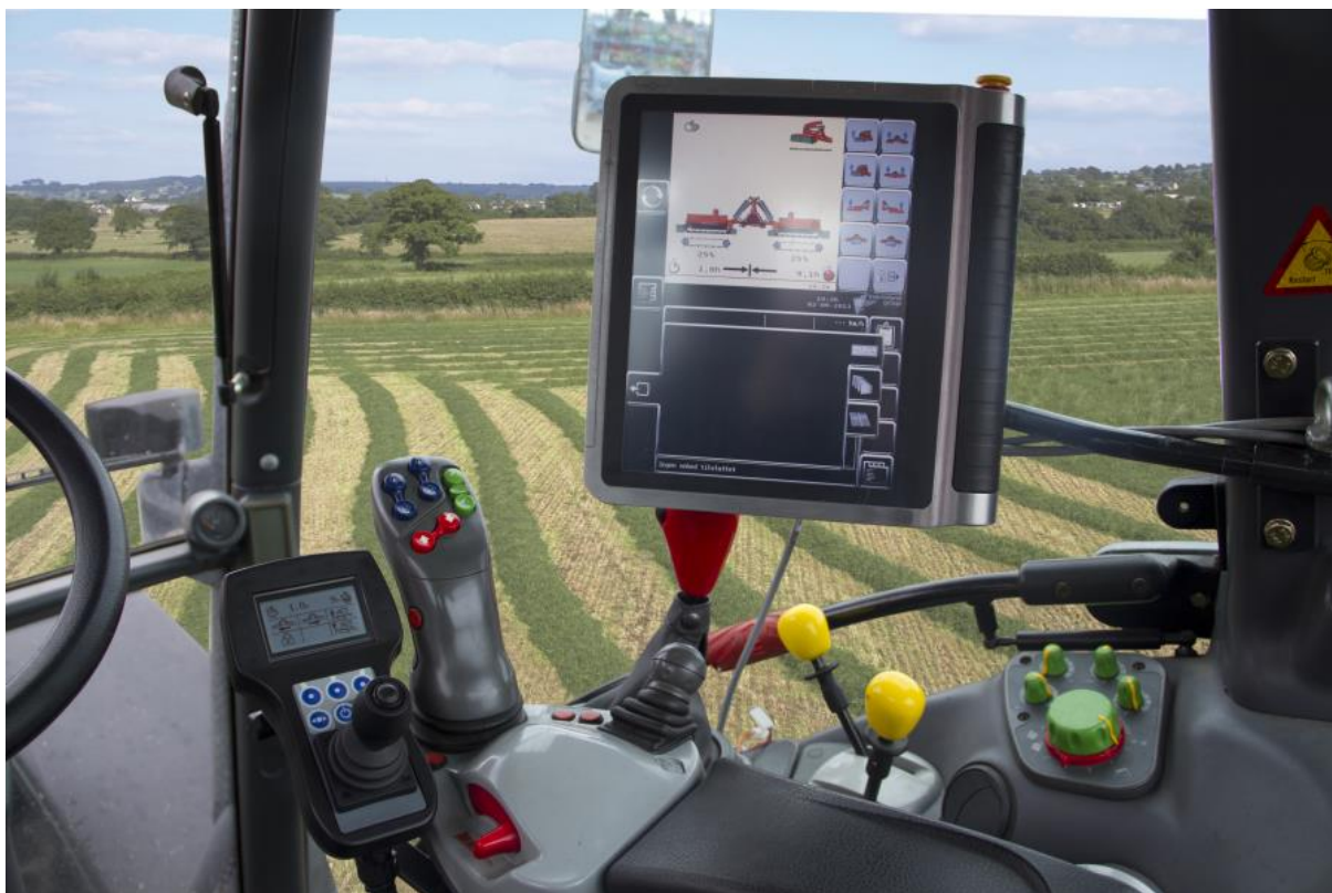
Joystick control positioned very conveniently in the tractor cab.
