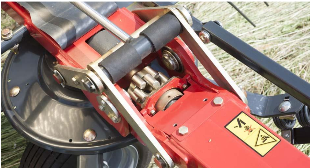
Vicon HexaLink finger clutch permits the rotors to fold 180° for transport
