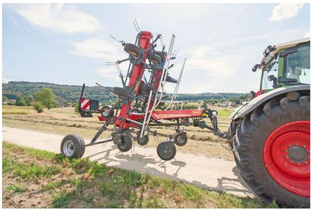
Compact transport dimensions. Despite 11.2m working width, the Vicon Fanex 1124 C offers a transport length of only 4,29 m
