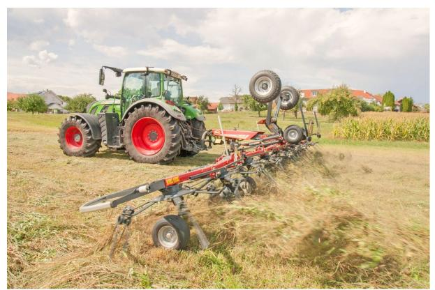
Vicon launches its new Fanex 1124C, an 11,2 m trailed rotary tedder that delivers high performance, short construction with modern design.
