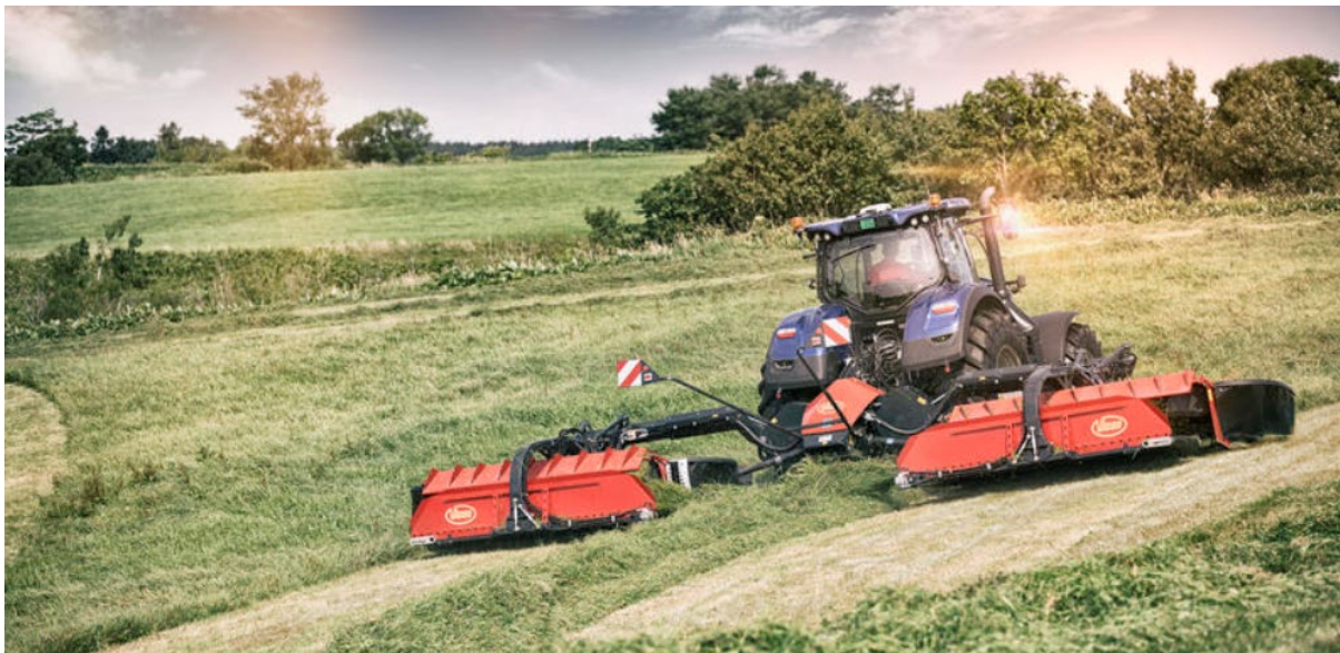
The new Vicon EXTRA 7100 BX triple mower with 10m working width and swath belts.
