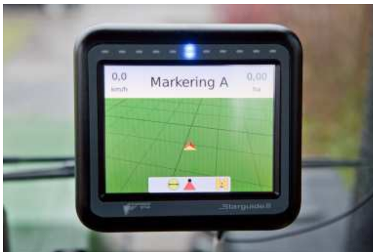
Starguide III automatic GPS section control
